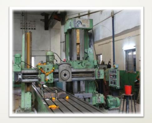
Plano Miller For Heavy Machining with table 900 mm x 8000 mm Long. Mono Column Admit 1000mm.
